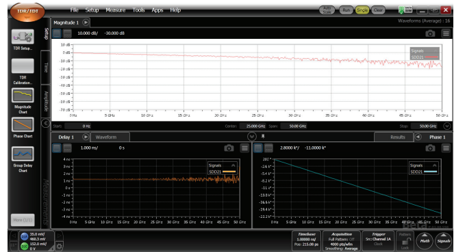
FlexDCA displays accurate S-parameter magnitude, phase and group delay plots simultaneously.
